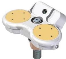
The system consists of a powered pressure and temperature sensor with transmitter fitted to a wheel rim, this sends pressure and temperature data over an RF link to a compact receiver on the car. Sampling rates increase automatically when a change in pressure is detected and the system shuts down below a threshold pressure to preserve battery life. The receiver sends data to the car control via CAN.
